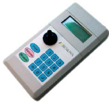
Fig. 5: Hand-held device for photometric detection of Senova mini columns
